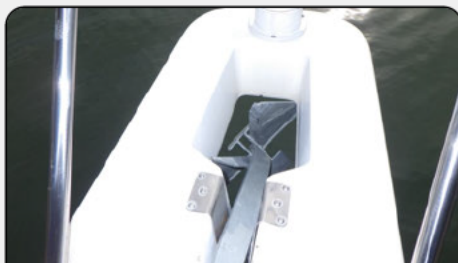
Photo 2: Note bend to port in the shaft as it enters the center of the anchor.
