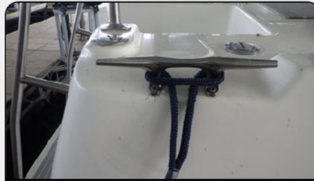
Photo 13: Cleat showing signs of cracking.
