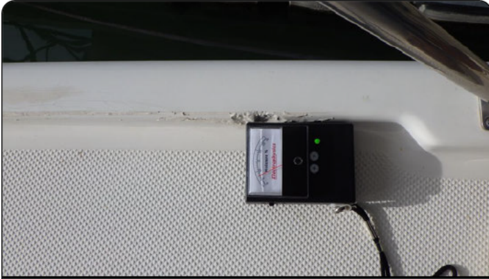
Photo 31: poor quality repair to toe rail but moisture level low
