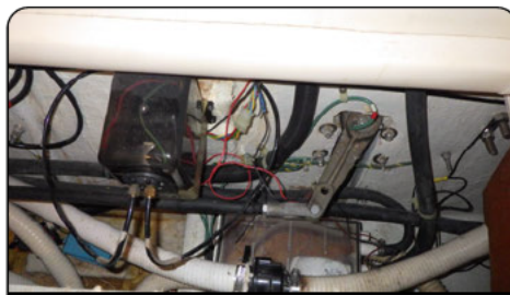
Photo 34: Steering hydraulics again but note good bonding wire to lever and general cleanliness
