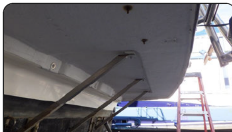
Photo 49: New swim platform support
